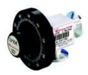
The LV10K needle valve provides fine control of gas bleed into a vacuum chamber or a regulated leak to control pressure in a vacuum system and is suitable for gas admission down to 10° mbar / 8 x 10° Torr. Suitable for pipeline or panel mounting.
