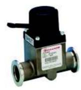
The IPVMK is a quick acting, bellows sealed, right-angled lever operated valve and is available with either an Aluminium or stainless steel body. The lever, connected to a self-lubricating plastic cam-piston, actuates the valve stem and valve plate through PTFE bearings. The valve plate O-ring groove is vented to prevent gas bursts. The valves are designed to operate down to  $10^{-9}$  mbar / 8 x  $10^{-10}$  Torr and up to a pressure of 2100 mbar / 1575 Torr (30 psi).
