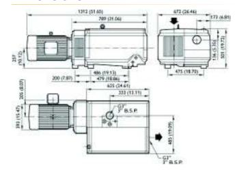
400 m<sup>3</sup>h<sup>-1</sup> / 241 ft<sup>3</sup>min<sup>-1</sup> Pumping speed 50 Hz 480 m<sup>3</sup>h<sup>-1</sup> / 289 ft<sup>3</sup>min Pumping speed 60 Hz Ultimate pressure without gas 0.5 mbar
