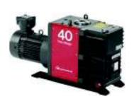
Edwards E2M40 series two stage oil sealed rotary vane vacuum pumps are renowned for their high ultimate vacuum, rapid pumping speeds, quiet operation and ability to handle water vapour. These direct drive rotary vane pumps are inherently compact and vibration free, and with their finger-proof fan and coupling housings they offer excellent operator protection.
